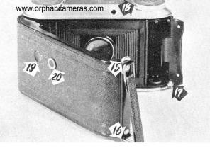
The camera back is opened by pressing the two catches (#15) and ( $\mp$ 16). The left spool chamber below the rangefinder knob holds the unexposed roll of film while the right one (#17) carries the empty take-up spool. Both roll holders swing out for convenient loading.
